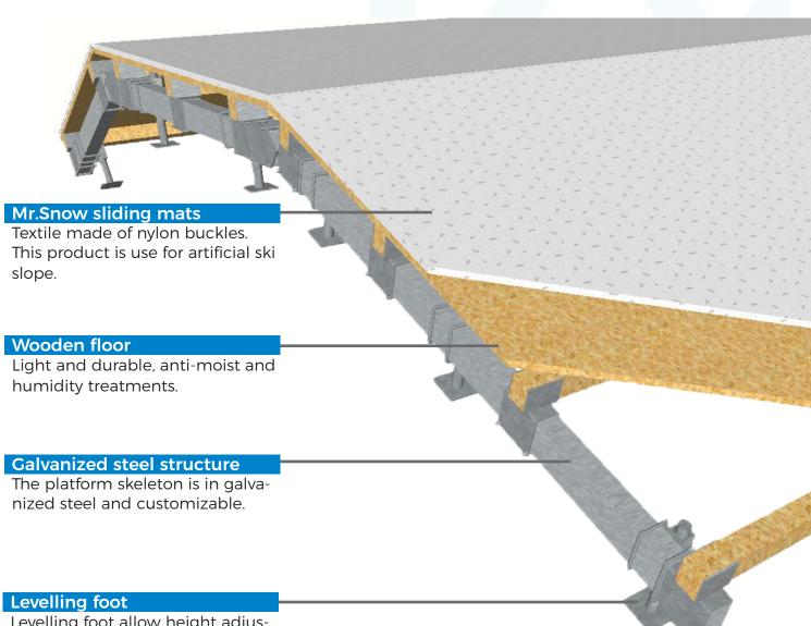
Levelling foot allow height adjustements and platform configuration changes (winter or summer use).
