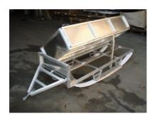
Developed in close collaboration with the operators of ski areas, sledges meet all needs and facilitate the transport of material and goods within the ski area
